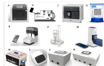
FIG 1 Point-of-care HIV viral load equipment and test cartridges currently marketed (A to F) or in development (G to K). Attendant key equipment for some devices, such as monitors, barcode scanners, or printers, is not included. (A) The Abbott m-PTiVA analyzer; (B) the Abbott m-PTiVA HIV-1/2 test cartridge; (C) the Cepheid GX4 instrument; (D) the Cepheid Xpert HIV-1 viral load test cartridge; (E) the DRIV SAMBA II test module with controller; (F) the DRIV SAMBA II plasma semiquantitative test; (G) the Cepheid Omni instrument and controller; (H) the Abbott Diagnostic Truempic sample preparation device; (I) to (K) the Abbott Diagnostics Truempic amplification instruments in Uno (I), Duo (J), and Quattro (K) module formats. (Images are reprinted with permission of the respective manufacturers.)
